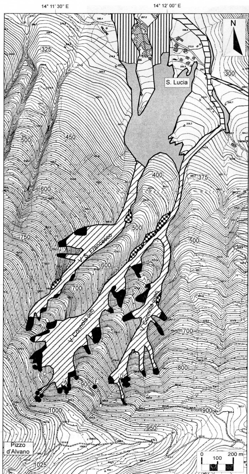
Figure 6. Zonation of the Connola - S. Francesco area. Legend: 1) Zone of detachment; 2) Zone of erosion - transport; 3) Zone of erosion - deposition; 4) Lateral landslide, showing retrogressive distribution of activity; 5) Zone of deposition; 6) Zone of canalization; 7) Location of the stratigraphic profiles (letters refer to Fig. 3).
