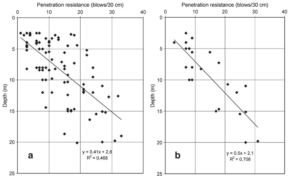
Fig. 16. Standard Penetration Tests of surficial deposits at Camaldoli hill: (a) overall plot; (b) tests performed at the upper reach of the main slope.
