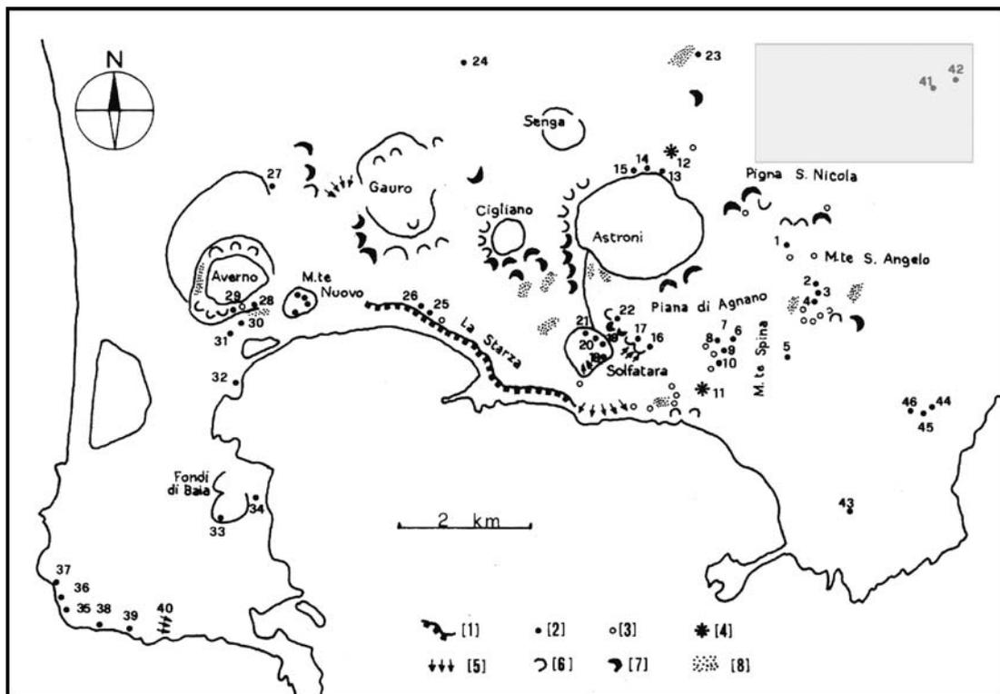
Fig. 10. Slope instability map of the Naples area (after Beneduce et al., 1988). Explanation: (1) terrace rim; (2) rapid earth flow; (3) debris slide; (4) earth slump; (5) rock fall; (6) areal erosion; (7) linear erosion; (8) shallow landslide. The inset refers to Camaldoli Hill.
