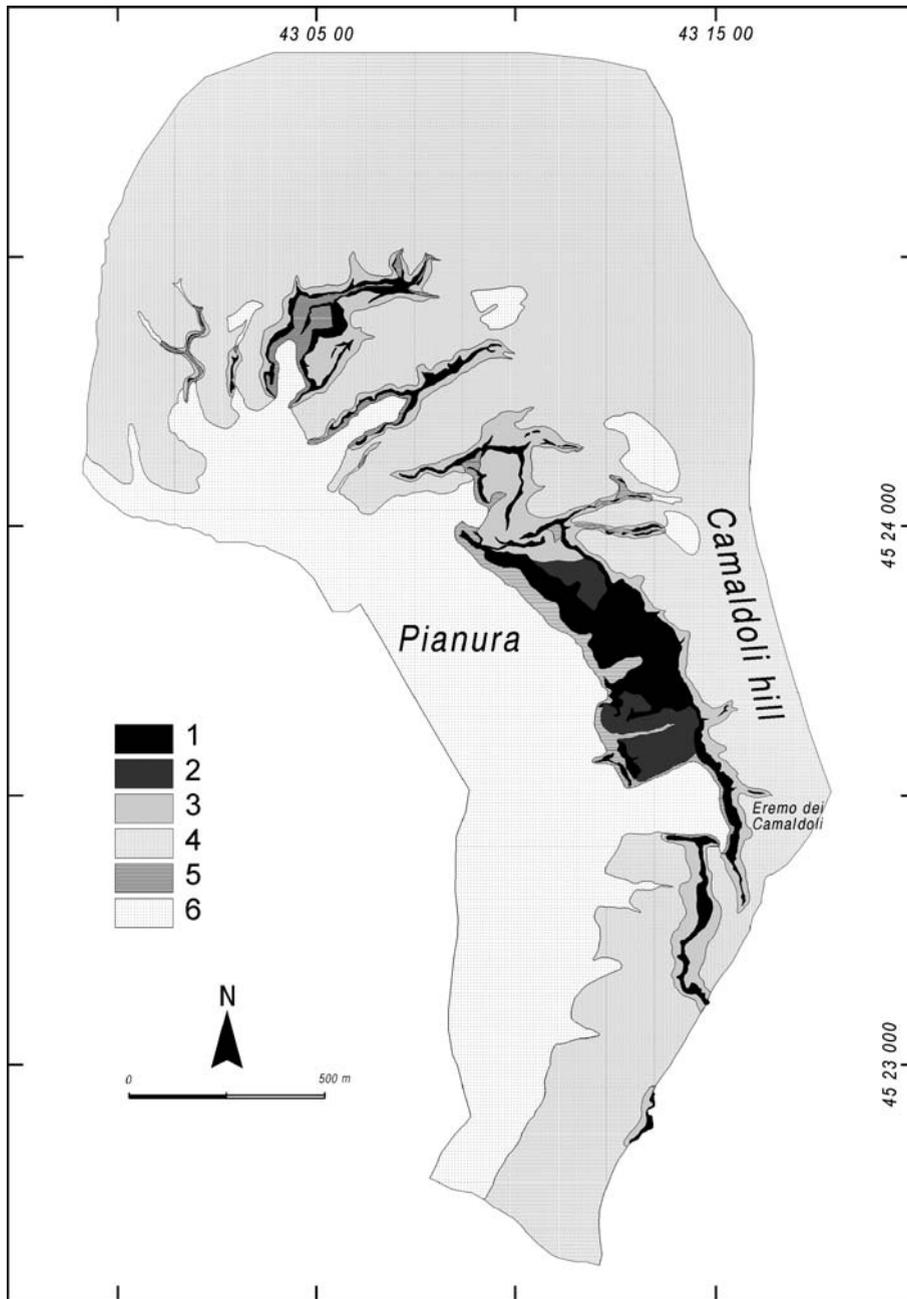
Fig. 6. Thickness map of loose deposits at the western slope of Camaldoli Hill. Pyroclastic sequences: class 1=0.0–0.5 m; class 2=0.5–1.0 m; class 3=1.0–5.0 m; class 4>5.0 m. Old landslide, slope, plain and valley-bottom and anthropogenic deposits: class 5=0.5–5.0 m; class 6>5.0 m.
