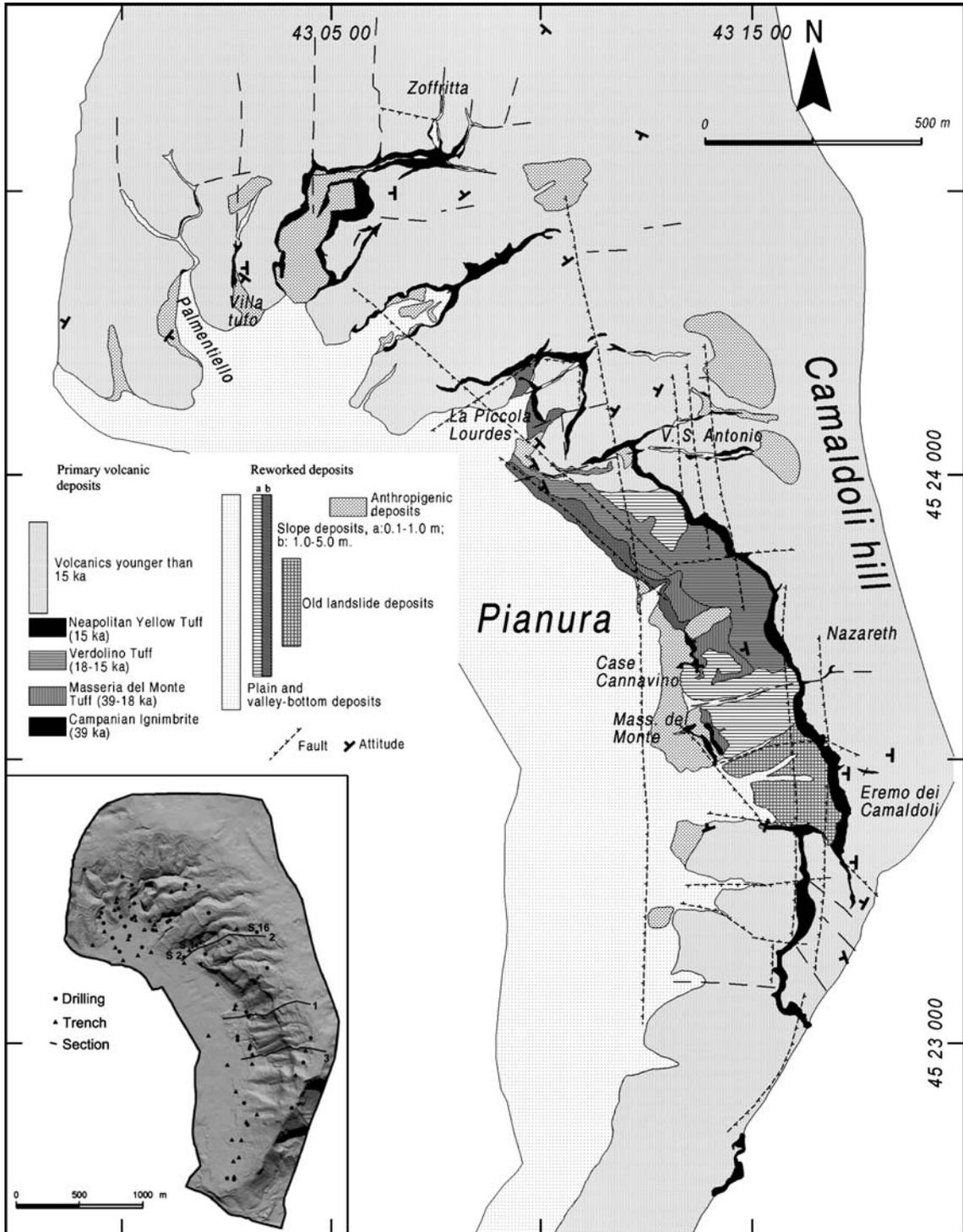
Fig. 3. Geological map of the study area. In the inset locations of boreholes, trenches, and cross sections are shown.
