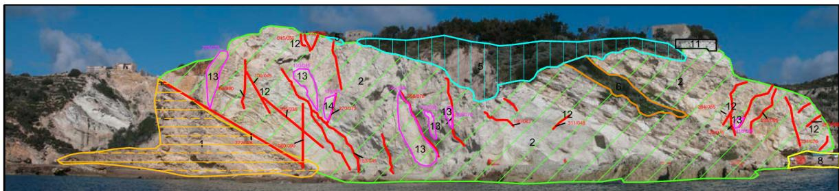
**Fig. 6 Geostructural photo-mosaic map at Cala dell'Acqua.** Key: 1) massive rhyolitic hyaloclastic deposit in breccia facies, with abundant glassy cement and coarse elements (L1); 2) massive rhyolitic hyaloclastic deposit in microbreccia facies (L2); 5) bentonite deposit (L5); 6) alluvial and colluvial deposits (L6); 8) beach deposits (volcanic gravel and sand) (L8); 11) anthropogenic material (L11); 12) main discontinuity and attitude (L12); 13) plane of discontinuity and attitude (L13).
