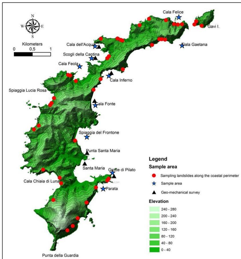
*Fig. 2. Location of the main landslides observed along the cliffs of Ponza Island, also showing the studied areas (Frontone, Fonte, Inferno, Gaetana, Felice, dell'Acqua, Feola, Lucia Rosa, Parata, Grotte di Pilato and Santa Maria).*
