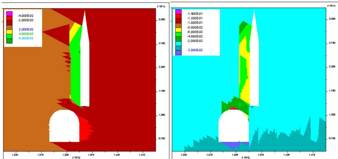
**Figure 13.** Contours of horizontal (left) and vertical displacements (right) due to the interaction between the oldtunnel and the karst chimney.
