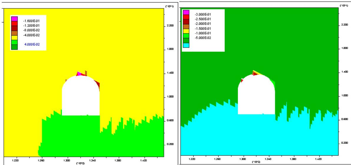
**Figure 12.** Contours of vertical displacements for joint friction angles  $\phi = 35^\circ$  and  $\phi = 45^\circ$ .
