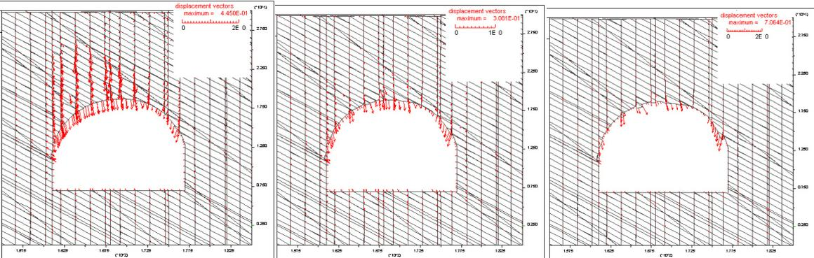
Figure 9. Block displacement vectors for different joint friction angles ( $\phi = 35^\circ, 40^\circ$  and  $45^\circ$ ).
