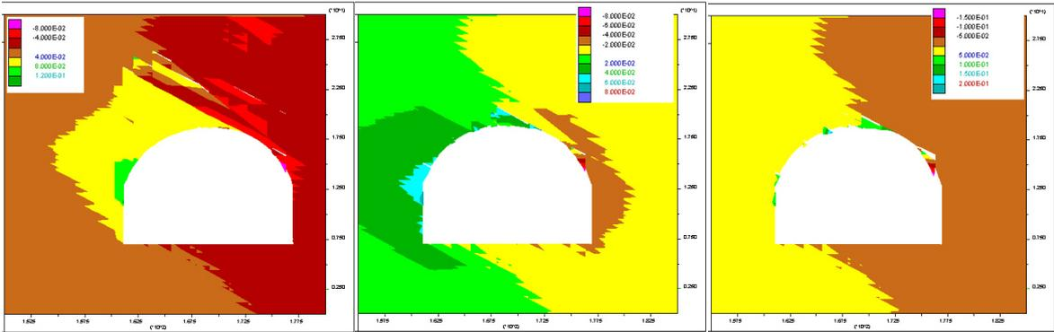
Figure 10. Contours of horizontal displacements for three different values of joint friction angles ( $\phi = 35^\circ, 40^\circ$  and  $45^\circ$ ).
