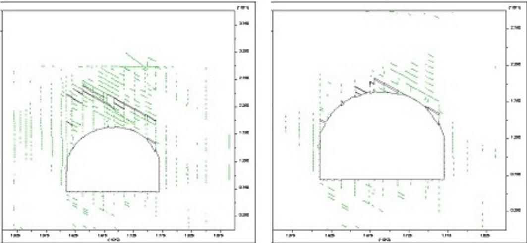
Figure 11. Joints subjected to zero normal stress for joint friction angle  $\phi = 35^\circ$  and  $45^\circ$ .
