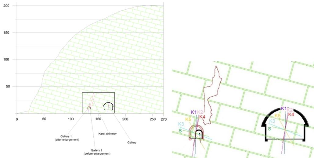
Figure 8. Cross section considered for the analysis, and close-up view with indication of the discontinuity sets.
