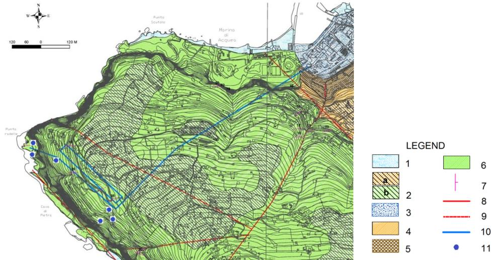
**Figure 1.** Geological map. Legend: 1) recent beach deposits. Holocene. 2) Indifferentiated pyroclastic deposits, resting over ignimbrite terraces (a) and low-gradient carbonate slopes (b). Holocene. 3) Alluvial fan deposits. Holocene. 4) Campanian Ignimbrite. Upper Pleistocene. 5) Ancient alluvial fan deposits. Upper Pleistocene. 6) Meta limestones. Cretaceous. 7) Strata bedding. 8) Fault. 9) Tectonic contact, dashed where presumed. 10) Trace of gallery. 11) Station for geosurvey.
